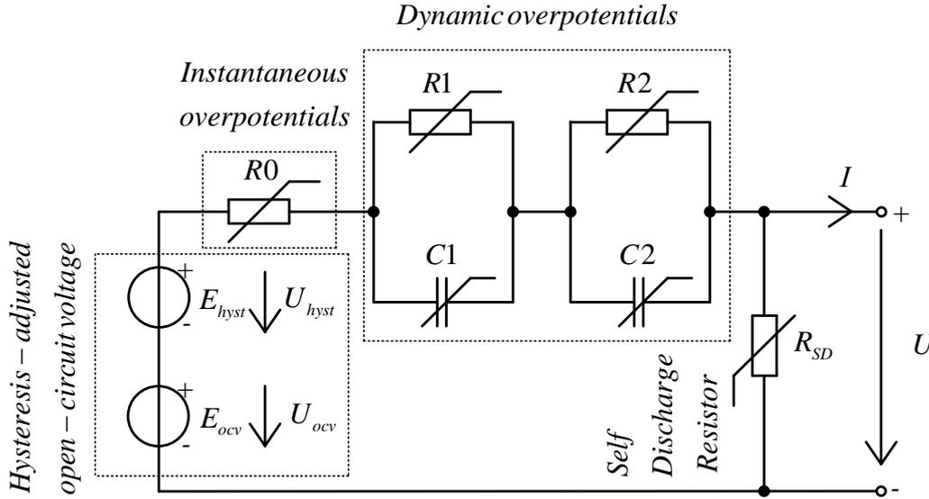
Figure 1 – Equivalent circuit diagram of battery
