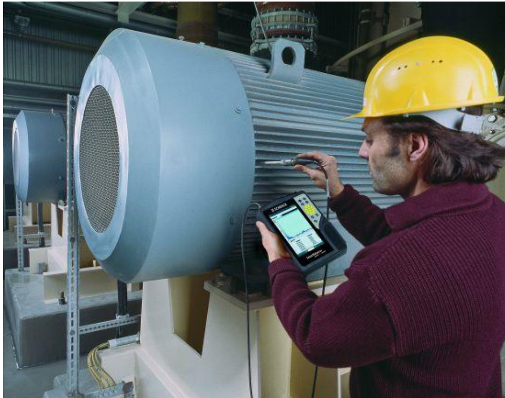
Figure 2 – The process of vibration diagnostics
