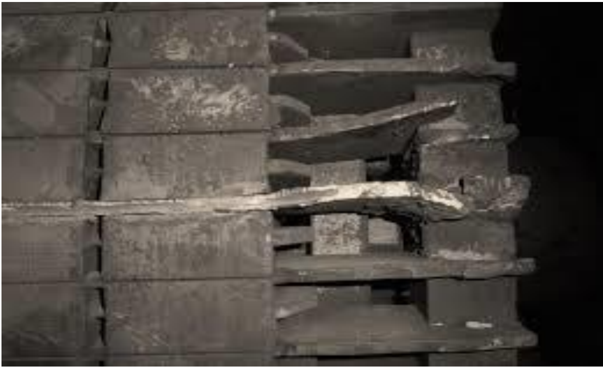
Figure 5 – Separation of rods from the short-circuited ring
