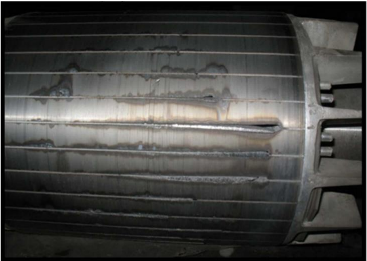
Figure 4 – Thermal damage of the rod of the SC rotor due to frequent restarts in the heated state.
