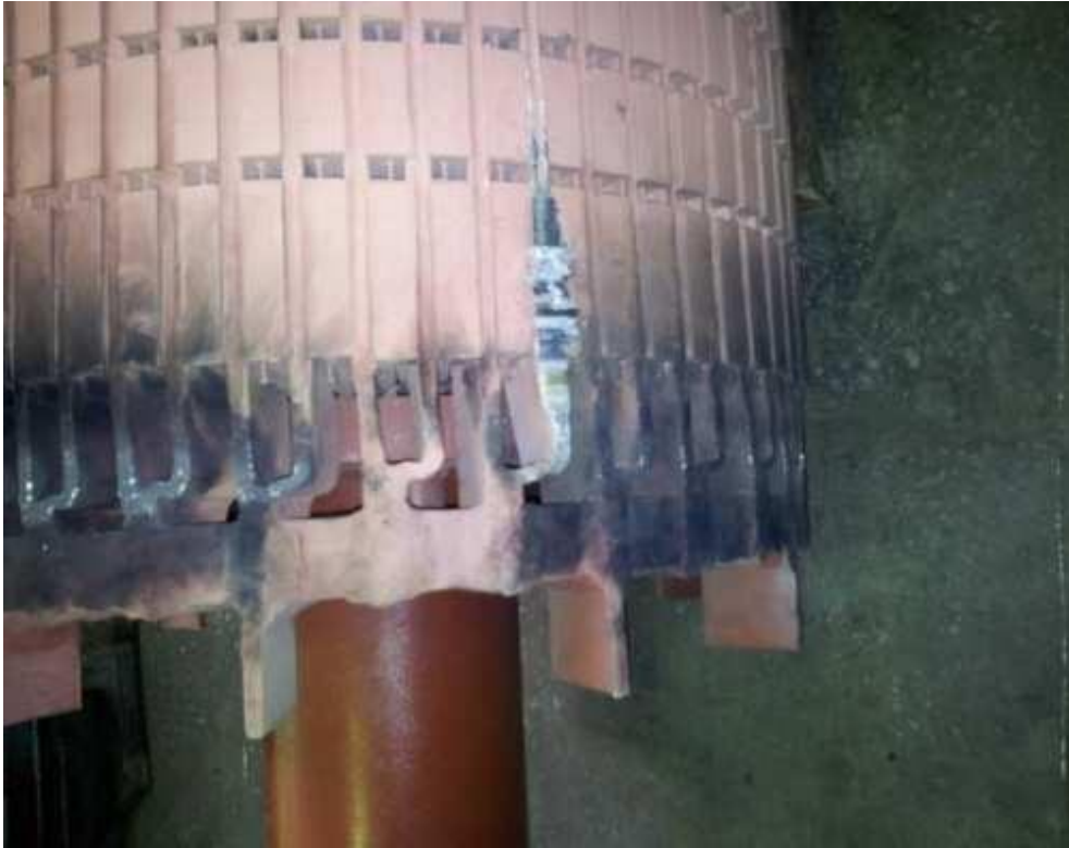
Figure 2 – The output of the rod from the slot due to the action of the electrodynamic forces when starting the motor
