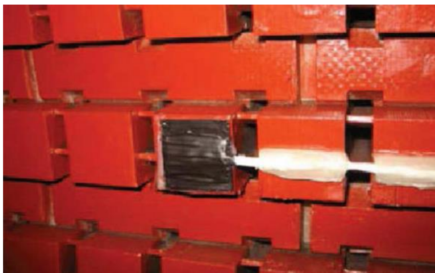
Figure 2 – Mounting a diagnostic coil on a stator tooth [2]
