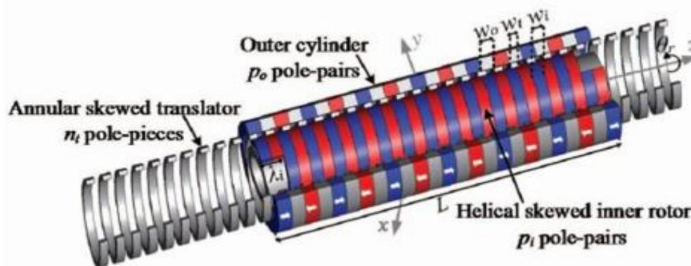
Figure 4 – MG lead screw
