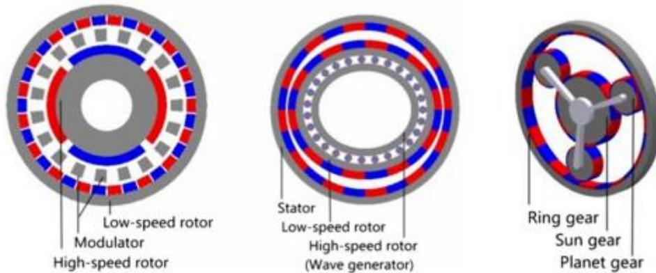
Figure 1 – Concentric, harmonic and MGs [5]
