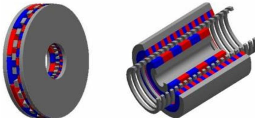
Figure 2 – Disc – type and linear type MG topologies [5]
