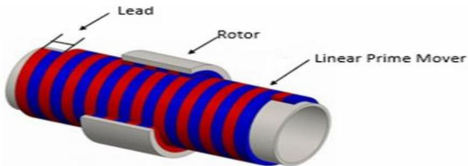
Figure 3 – Magnetic lead screw
