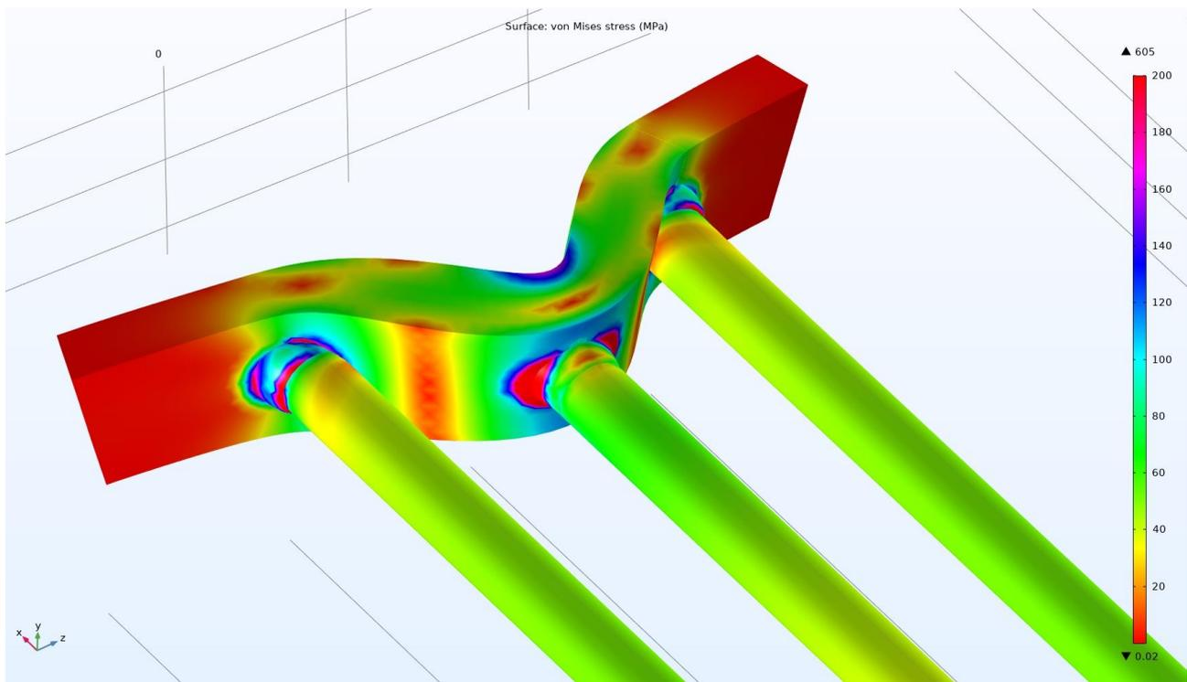
Figure 1 – Distribution of thermomechanical stresses in the SSCR and the rods of the DW with the presence of SE of the rotor  $\varepsilon = 0,83$  (view from the core of the pole)
