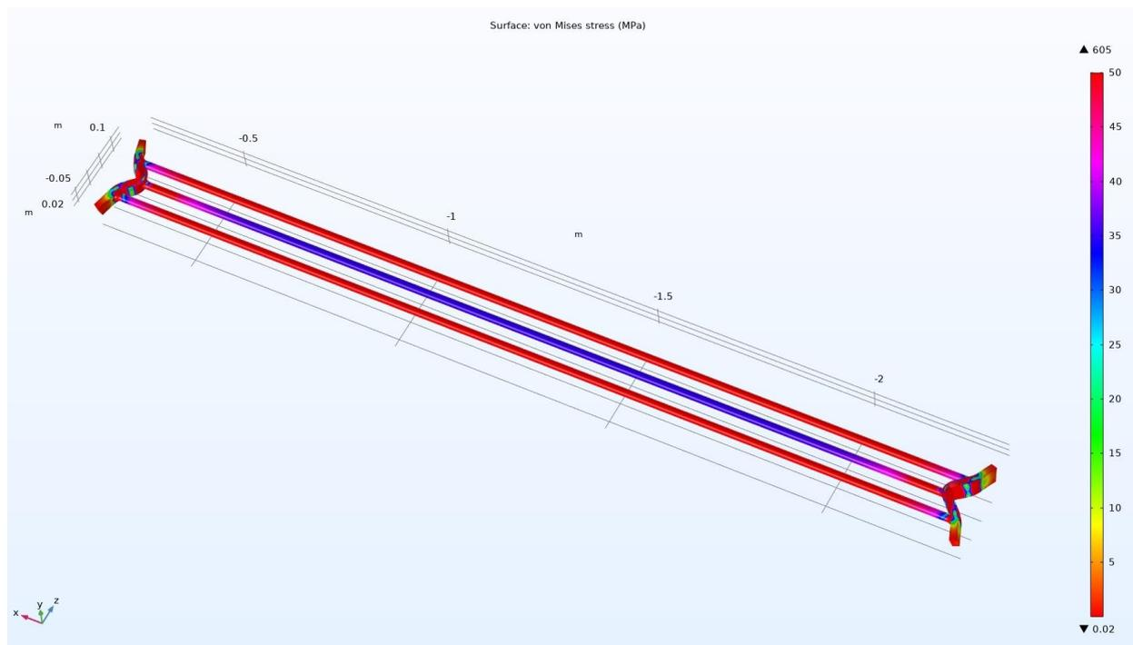
Figure 3 – Distribution of thermomechanical stresses in DW rods with the presence of SE of the rotor  $\varepsilon=0,83$
