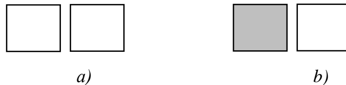
Figure 2– Scheme of two transformers with a power of 1000 kVA: a) normal mode; b) emergency mode; disabled transformer is shown in dark
